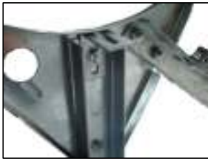
The L shape adapters are used to tighten and safe the tank on the support base.
