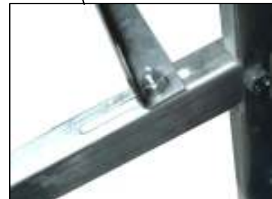
In the same way the collector's L supporters are fixed on the top of the support base to hold the collector
